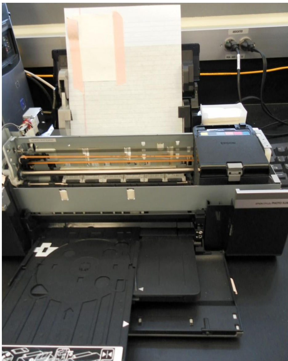
Figure 2. EPSON R280 inkjet modifications for printing carbohydrate bio-inks; uncovered printing mechanism including cartridges, inkjet, and DVS-activated sheet taped onto normal printer paper, ready to be printed with bio-ink.
